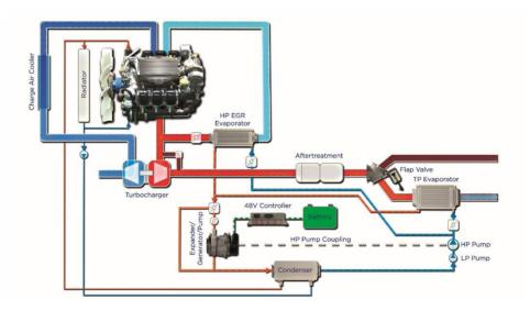
BorgWarner's ORC waste heat recovery system enables improved fuel economy by converting waste heat into electrical energy.
