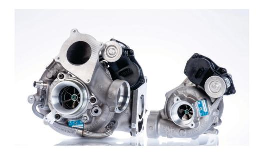
BorgWarner's regulated two-stage turbocharging technology with two VTG turbochargers boosts performance and transient behavior of numerous BMW Group models while contributing to improved fuel economy and reduced emissions.
