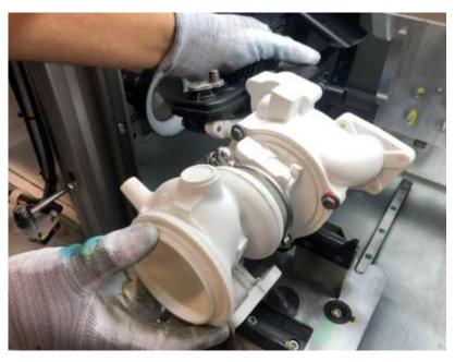
3D prototyping enables optimized efficiencies and precision for assembly, changes needed before entering the production line and simulated assembly tests in the engine.
