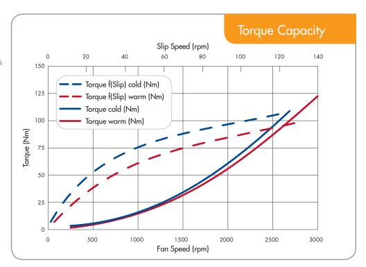
Since the centrifugal forces and the silicone fluid viscosity are mainly responsible for the flow rate of the fluid through the fan drive, the response behavior is mainly dependent on these two parameters.
