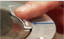
Worn lining – replacement required. Notice how the tool protrudes above surface of the lining retainer plate.
