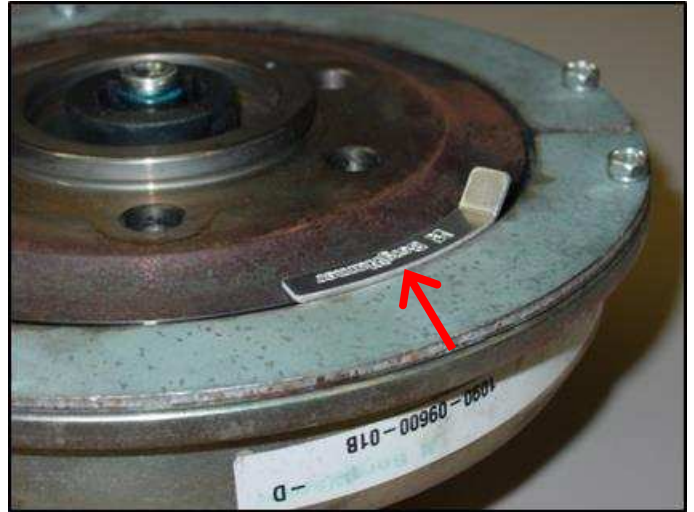
Liner Replacement Necessary
