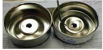
This type of failure is caused from an object coming in contact with the front of the clutch. The damage bends the piston/cylinder cap and causes an air leak. In some cases it will prevent the clutch from engaging or only allow partial engagement. This is not warrantable.
