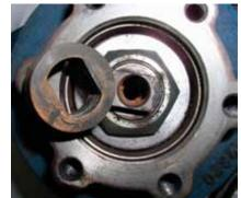
Contamination in the system may cause clutch failure, seal leaks, and operation problems. This failure is not warrantable.
