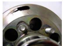
If a clutch mounting bolt is not properly torqued and comes out or a bolt is dropped into the housing and not removed, the failure above may occur. This is not warrantable on service parts or if the clutch and hub have been separated for service or repair.
