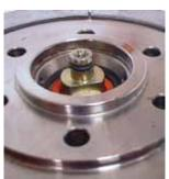
Damage to the base of the piston rod or o-ring is caused by a hub (pulley and bracket) problem. If this is the case, the hub must be under warranty and accompany the clutch in order to be warrantable.
