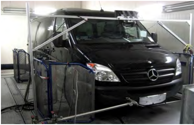
Mercedes-Benz Sprinter in climatic test bench, OM642 cooling system
